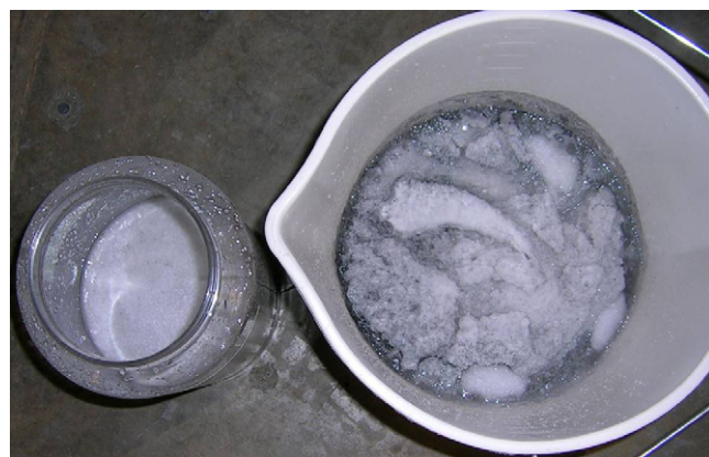
Fig. 10. Discharge products (left for 20% solution and right for 15% solution).
